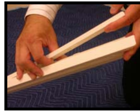
Slide finger along frame to safely release the filler strip.
