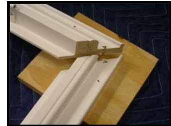
Position the left frame on the Hoffman Key and push down until the frames mitered edges are flush.
