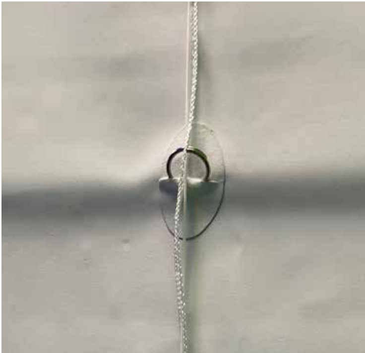
Patch Covering Pinholes Made When Sewing On Cord Rings
